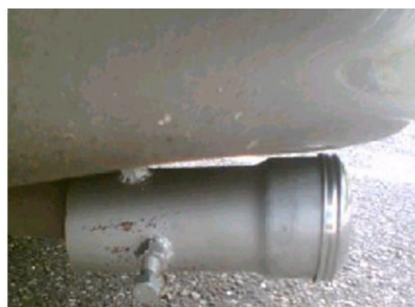
Sample collector coupled to motor vehicle's exhaust pipe
