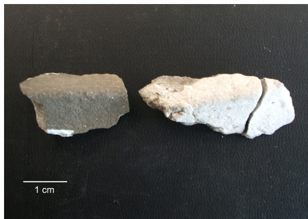
Fig. 7. Appearance of a sample after the cleaning treatment in comparison with a sample having the initial black crust on the surface.
