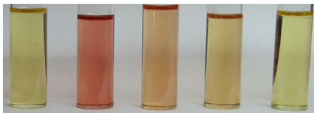
Fig. 2. Color changes of 1 ( 2 \times 10^{-5} M) upon addition of 8 equiv. of different anions in DMSO:H 2 O (95:5, v/v) mixtures at 298.2 \pm 0.1 K (from left to right: 1 only, 1 + \text{AcO}^- , 1 + \text{F}^- , 1 + \text{H}_2\text{PO}_4^- , 1 + \text{Cl}^- , \text{Br}^- , \text{I}^- ). (For interpretation of color in this artwork, the reader is referred to the web version of the article).
